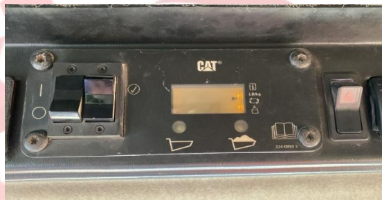
Gamabar 2.5 Monitor Payload Measurement System HD Cat
