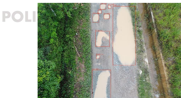
Gambar 3. 10 Hasil Deteksi Objek ( Potholes )
