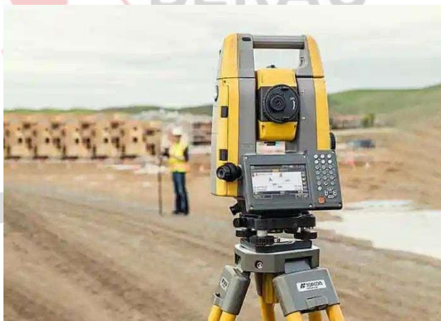
Gambar 2. 3 Alat Total station (Sumber: Mahajan, 2021)
