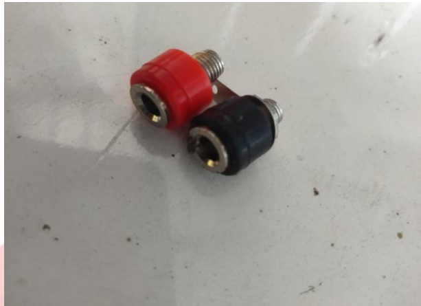
Gambar 2.26 Banana Jack Female 4 mm (Sumber, Dokumentasi Pribadi)
