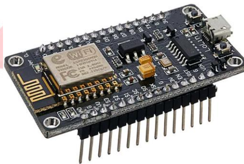
Gambar 2. 2 NodeMCU V3 ESP8266 (Rifaat & Sephiani, 2024)
