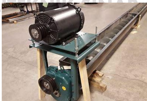
Gambar 2.6 Screw Conveyor (Sumber google)
