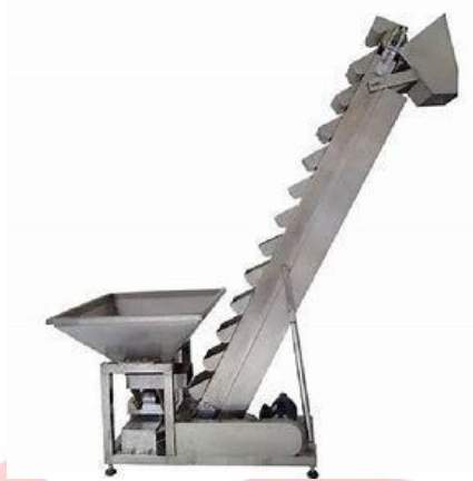
Gambar 2.7 Bucket Conveyor (Sumber google)
