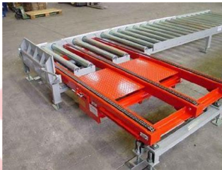
Gambar 2.5 Chain Conveyor (Sumber google)
