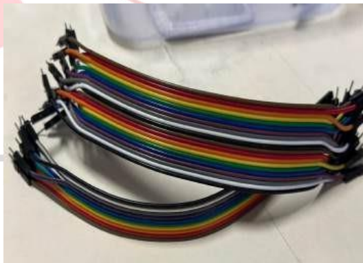
Gambar 2. 8 Kabel jumper (Sumber pribadi)
