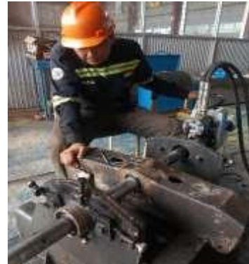
Proses line boring
