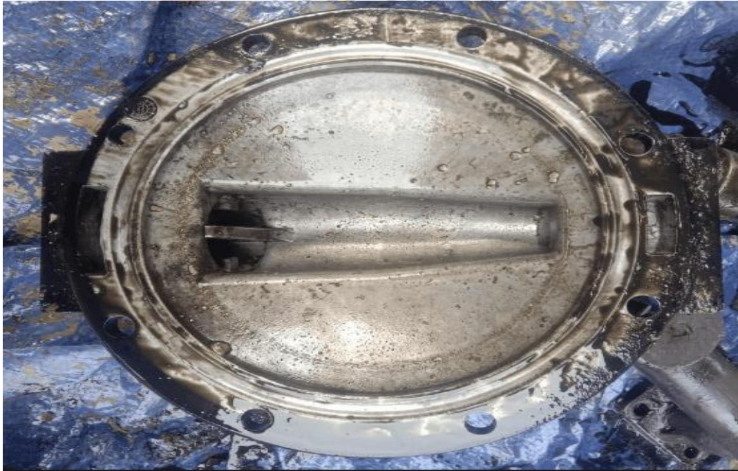
Lampiran 2 Kondisi Fluid Cover Diaphragm Pump Left
