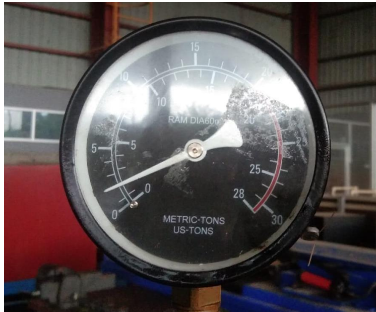
Lampiran 15 Pressure Gauge Penekanan Benda Uji B 1
