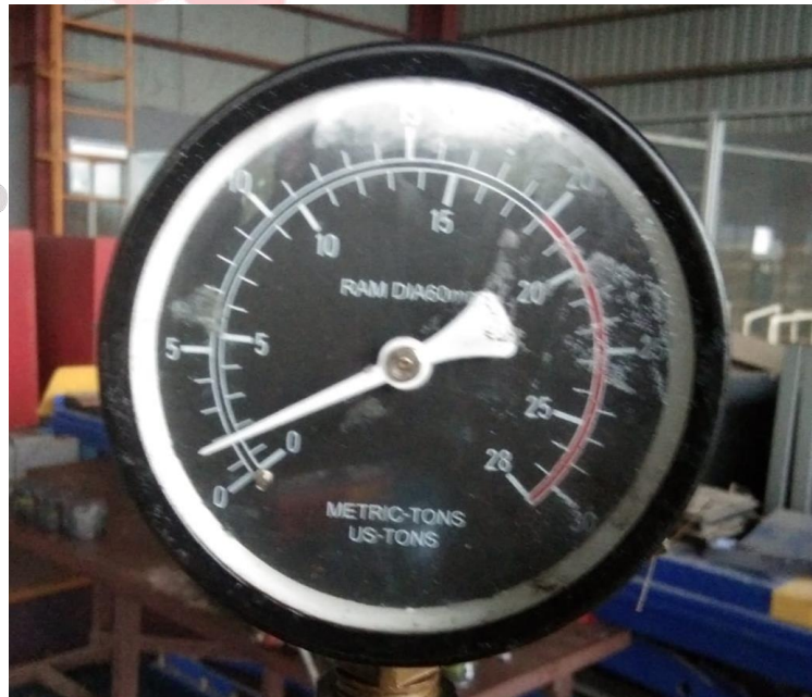
Lampiran 18 Pressure Gauge Penekanan Benda Uji B 2
