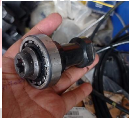
Gambar 2.7 Bearing Original (Spherical Roller Bearing) Sumber : Dokumentasi Pribadi (2022)
