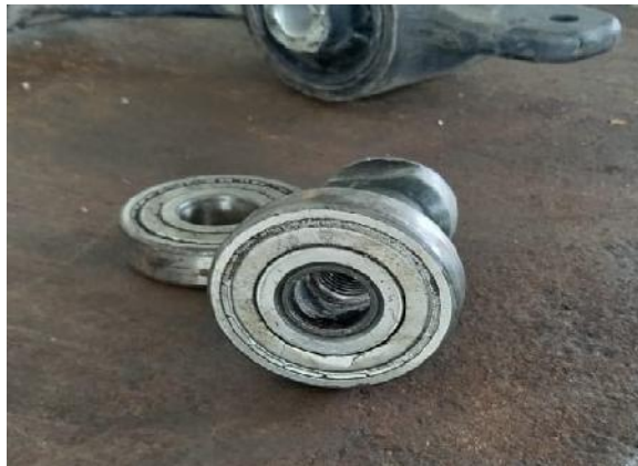
Gambar 2.8 Bearing After Market (Deev Grove Ball Bearing) Sumber : Dokumentasi Pribadi (2022)
