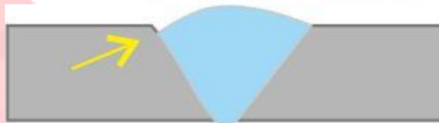
Gambar 2.10 Cacat Las Lack of Fusion Sumber : https://www.expertlas.com/cacat-las/#:~:
