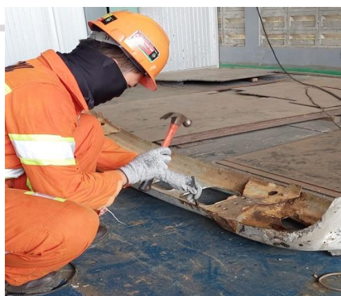
Proses Punch and chisel bumper
