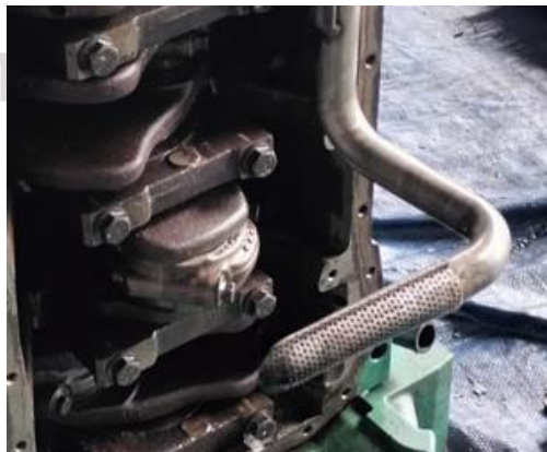
Gambar 2.8 Oil Strainer (Sumber: Dokumentasi Pribadi)
