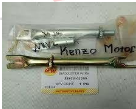
Gambar 2.13 adjuster brake Sumber : tokopedia.com.
