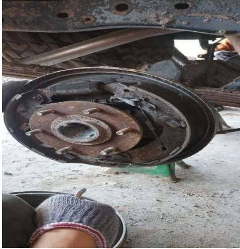
Gambar 15 sampel tromol kotor
