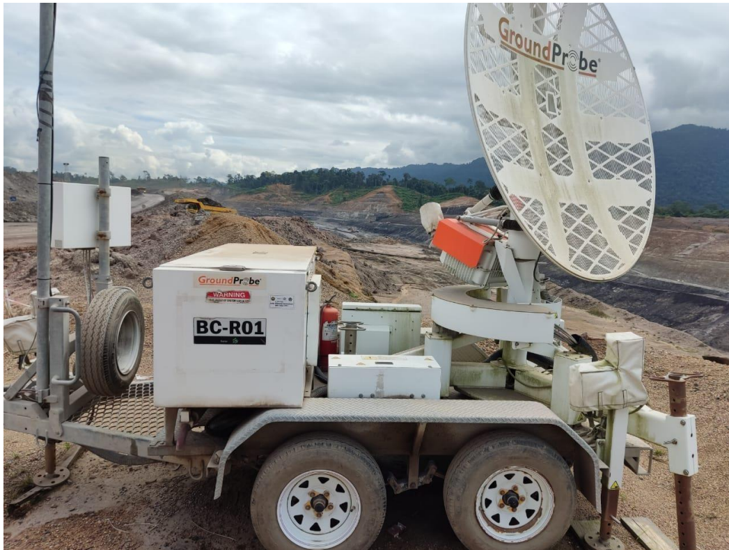
Gambar 3.2.1 Slope Stability Radar SSR-XT
