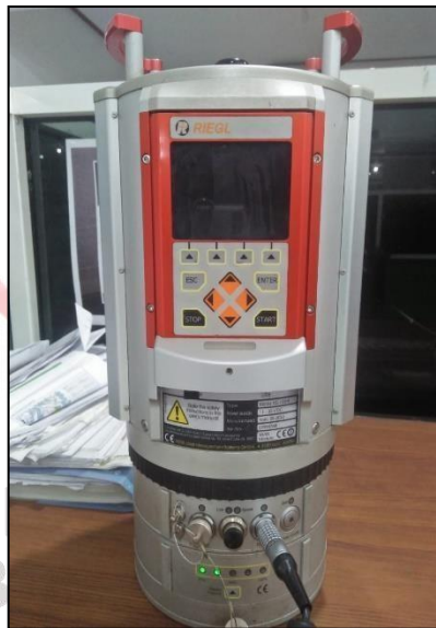
Gambar 2. 5 Laser Scanner (sumber PT. Berau Coal)
