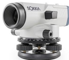
Gambar 2. 12 Sipat Datar ( Waterpass ) B40A, (Indosurta Group)
